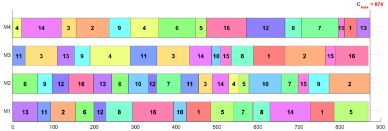
Figure 9. The optimal schedule of Instance 5 with 16 jobs by Jain et al. (2006).
