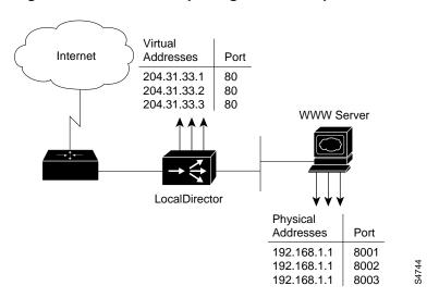
Figure 155 Forward Multiplexing Mode Example
